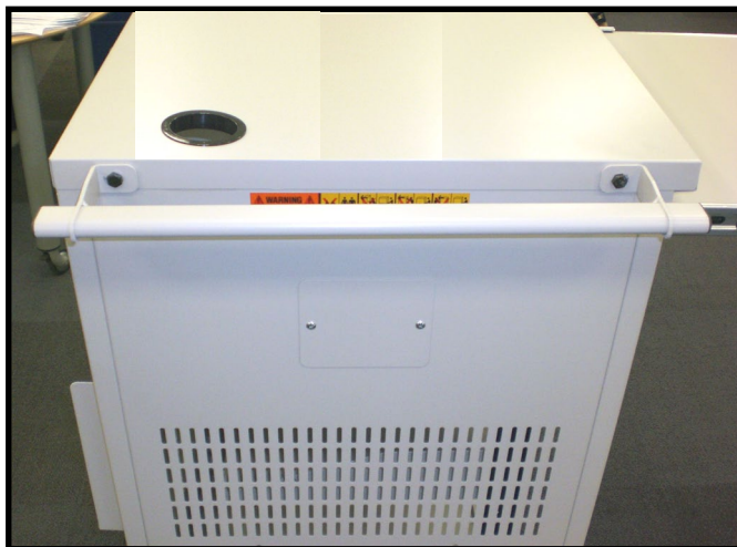
STEP 2: Attach handle with screws (AA) and nuts (BB).
