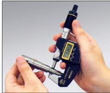
Measuring coaxial workpiece
