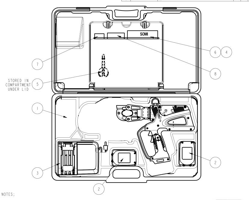
I. TOOL ACCEPTS 18V MAKITA LITHIUM ION BATTERIES, BL SERIES OF SIZE 2.0 AHR AND GREATER IF THE PLASTIC BATTERY CLIP IN THE TOOL HAS A "STAR" MOLDED INTO IT. THE "STAR" IDENTIFIES ACCEPTANCE OF THE BL SERIES BATTERIES
