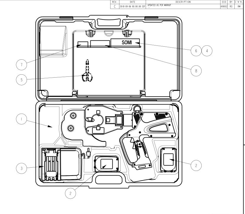
2. TOOL ACCEPTS 18V MAKITA LITHIUM ION BATTERIES, BL SERIES OF SIZE 2.0 AHR AND GREATER IF THE PLASTIC BATTERY CLIP IN THE TOOL HAS A "STAR" MOLDED INTO IT. THE "STAR" IDENTIFIES ACCEPTANCE OF THE BL SERIES BATTERIES.
