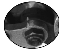
CORRECT: Index Marks Line Up
