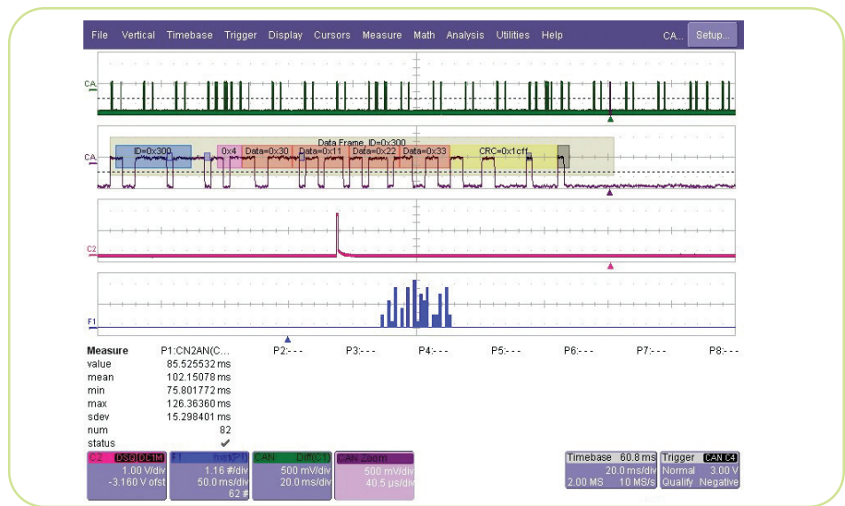
Figure 3. Using the CANtoAnalog parameter to determine sensor latency
