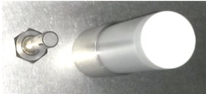
Figure 10: Plugged-in CO 2 sensor (right) and gas mixing head for CO 2
