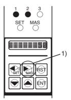
In Set-up Mode, hold down the right arrow (MAS) key for at least two seconds.
