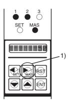
In Measuring Mode, hold down the right arrow (MAS) key for at least two seconds.
