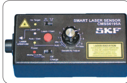
CMSS 6195A self-powered sensor with smart laser tachometer
