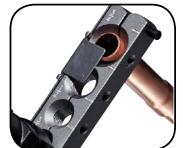
Slide gauge for perfect tube alignment before flaring
