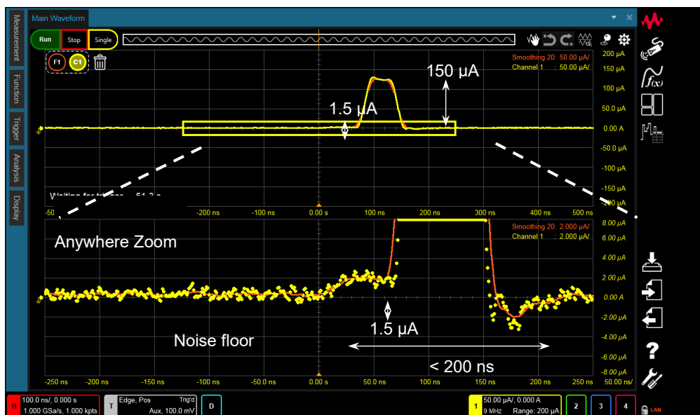
Figure 22. Pulsed measurement example using the pulse generator and CX3300A
