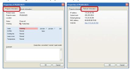
Projector name, location, status, lamp replacement, air filter cleaning and replacement information are displayed in the [Projector information] tab. The value in [Lamp time converted] is shown considering its duration. The sum of [Lamp time normal] and [Lamp time quite mode] is the total lamp usage time.
