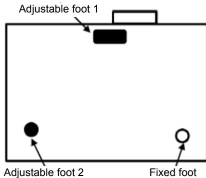
Diagram 1 shows the projector base, featuring two adjustable feet. Adjustable foot 1, located below the lens, is used to adjust the angle of the projector by raising or lowering the front. Adjustable foot 2 is used to adjust left/right tilt.
