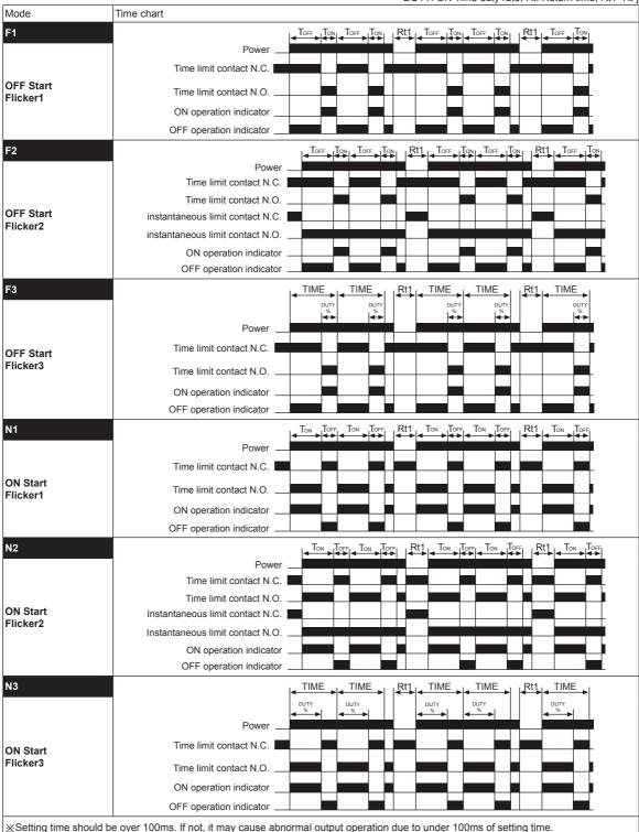
※[F3], [N3] mode operates flicker by setting cycle (time) and ON duty (%). ON time range changes to cycle (time) range and OFF time
