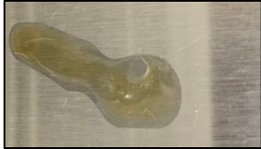
Rosin based flux on stainless steel test coupon
