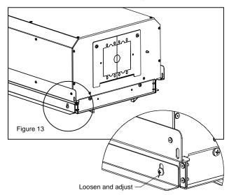
**NOTE:** Remove the cleat entirely to allow the enclosure to be mounted closer to the tile grid frame.
