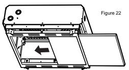
Push panel assembly back into place and rotate latches to lock position.
