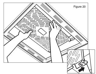
(4) Hand tighten nuts (I) to secure shelf in place.
