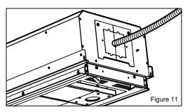
5 Attach complete outlet box configuration to projector mount plate as shown below in figure 12. Secure by re-attaching nuts removed in Step 1.
