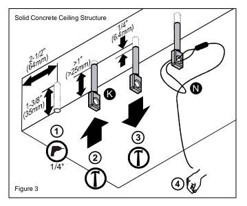
(2) Tap anchor (K) into each hole to a depth of at least 1" (25mm) (See Figure 3).
