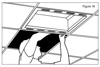
(2) Attach cables as shown (figure 17) using cable locks (L) to secure cable, adjusted to proper length - allowing box to be level, and NOT RESTING ON CEILING FRAMEWORK.
