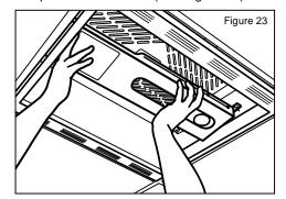
(2) Once into position, drop plate down onto mounting rails.
