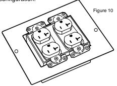
If outlet box configuration is attached to wiring/conduit prior to box attachment, remove two-piece electrical plate from box sidewall, feed configuration through large opening. Then re-attach two-piece plate to close around conduit.
