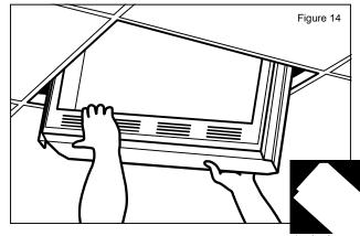
chamfered corners for easy clearance
