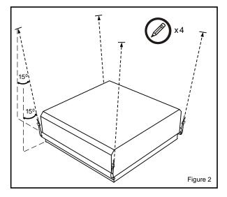
Examine ceiling structure (solid concrete, wood or steel truss) above kit to be installed to identify four support cable anchor locations. Each location should be approximately 15° outside of support holes in kit assembly. Mark locations with a pencil.
