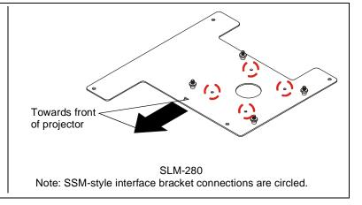
**NOTE:** Specific to SSB-style and SSM-style interface bracket installation: All appropriate screws come pre-installed in the circled locations above. DO NOT attempt to substitute and USE ONLY this pre-installed hardware for SSB-style and SSM-style interface bracket
