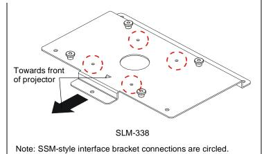
NOTE: Specific to SSB-style and SSM-style interface bracket installation: All appropriate screws come pre-installed in the circled locations above. DO NOT attempt to substitute and USE ONLY this pre-installed hardware for SSB-style and SSM-style interface bracket installation.
