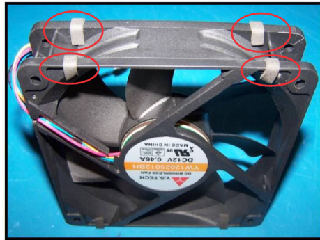
Figure 4 Foam Pad Placement - Opposite Side
