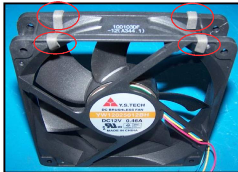
Figure 3 Foam Pad Placement
