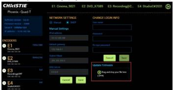
3. Configure the Encoder sources using the Phoenix Quad-T Web Manager.
