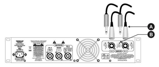
A 3-pin XLR, or 6.3 mm (1/4 in.) phono jacks connected to the CH. A and CH. B INPUTS
