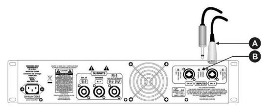
A 3-pin XLR, or 6.3 mm (1/4 in.) phono jacks connected to the CH. A INPUTS
