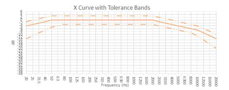
• Vive Audio line array target curve: developed for response of line array systems in cinema
