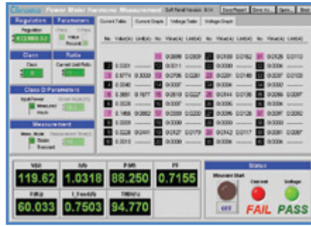
IEC 61000-3-2 Current Harmonics Test (Pre-compliance)
