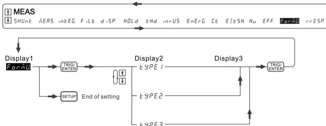
Figure 4-73 Process for Setting Formu
