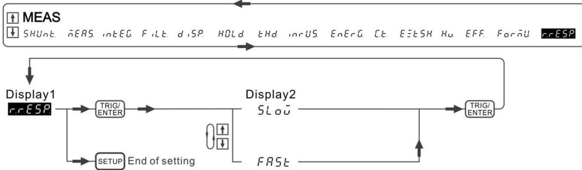
Figure 4-75 Process for Setting R.RESP
