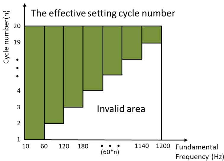
Figure 4-52 Effective Setting Cycle Number for Fundamental Frequency
