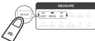
2. Use **↑**, **↓** to select HV function in 1<sup>st</sup> display window and press **TRIG/ENTER** to confirm it.
