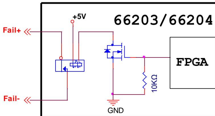
Figure A-3 Fail + / Fail – Internal Wiring Diagram
