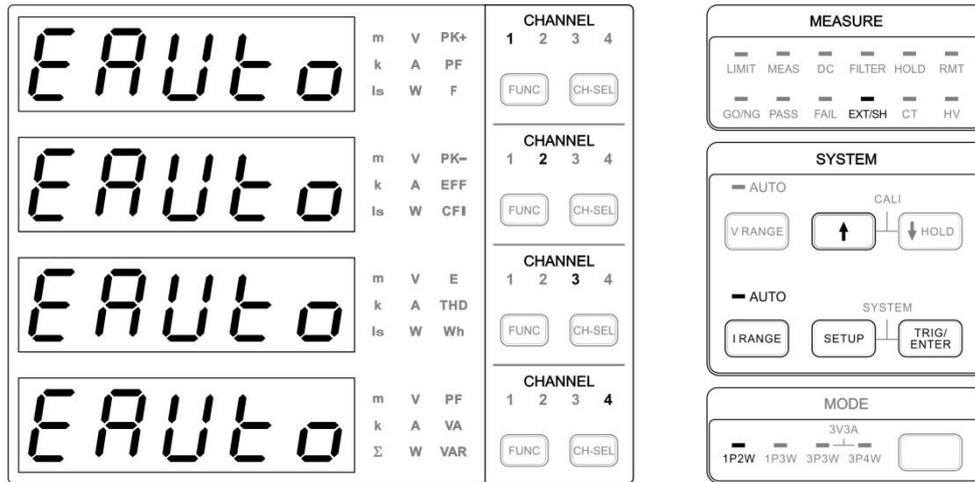
Figure 4-27 External Range Setup Screen
