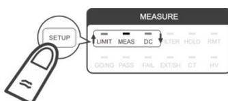
2. Use  $\uparrow$ ,  $\downarrow$  to select C.t. function in the 1<sup>st</sup> display window and press **TRIG/ENTER** to confirm it.
