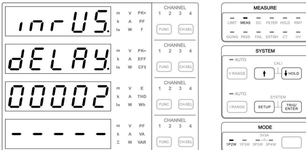
Figure 4-54 INRUSH CURRENT Setup Screen
