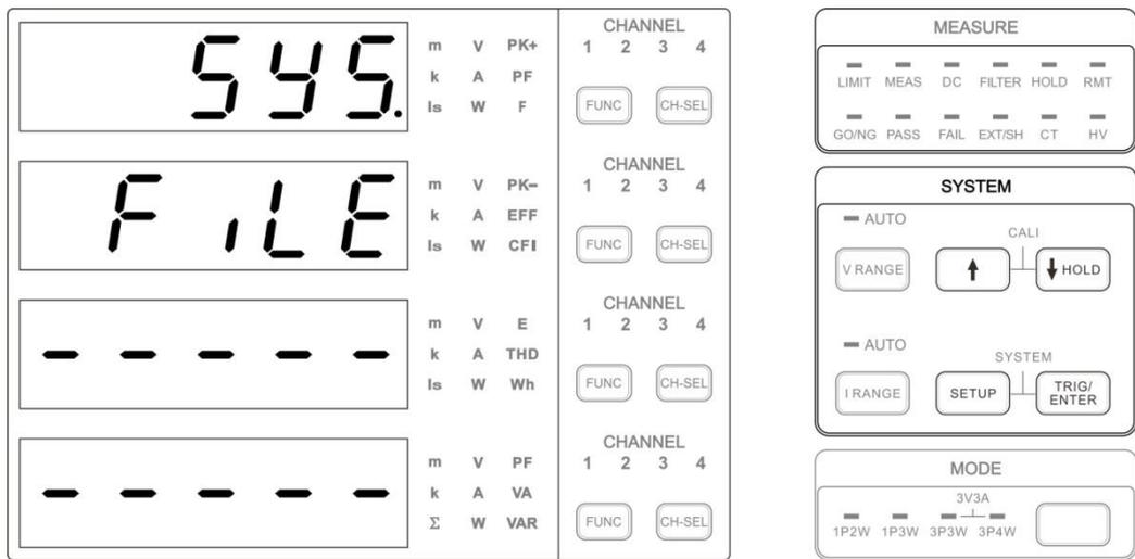
Figure 4-7 Menu for Storing & Recalling Setting File
