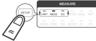
2. Use  $\uparrow$ ,  $\downarrow$  to select R.RESP function in the 1<sup>st</sup> display window and press **TRIG/ENTER** to confirm it.
