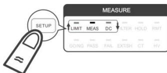
2. Use **↑**, **↓** to select ExtSH function in 1<sup>st</sup> display window and press **TRIG/ENTER** to confirm it.
