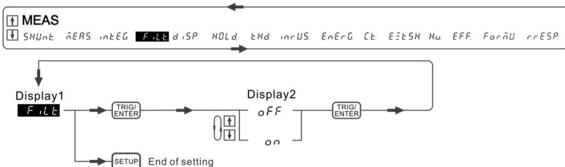
Figure 4-46 Process for Setting FILTER
