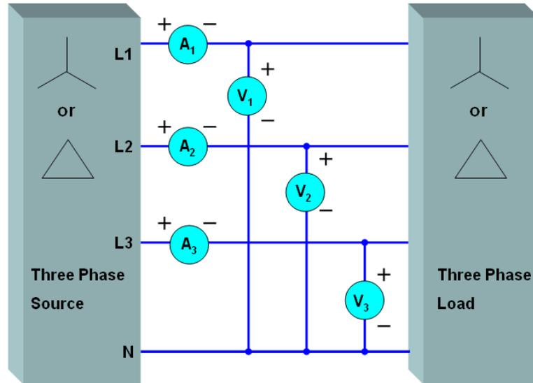
Figure 4-82 Three-Wattmeter Method Wiring
