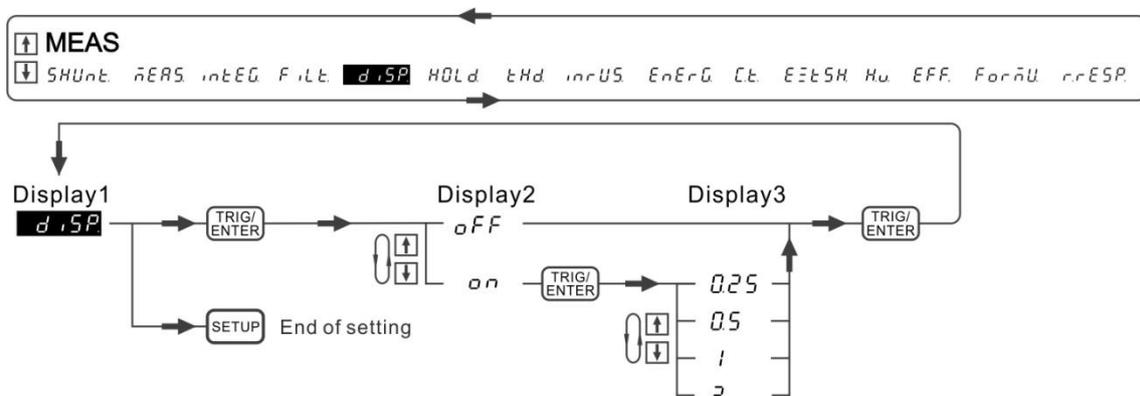
Figure 4-48 Process for Setting DISPLAY Refresh Rate
