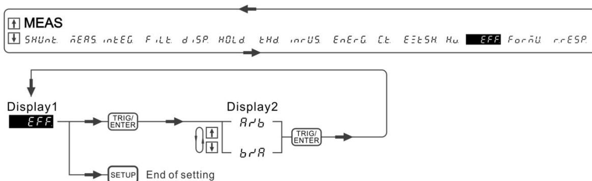
Figure 4-71 Process for Setting EFFICIENCY
