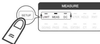
2. Use **↑**, **↓** to select THD in the 1<sup>st</sup> display window and press **TRIG/ENTER** to confirm it.
