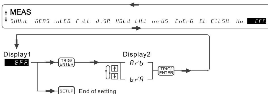
Figure 4-18 Process for Efficiency Calculation
