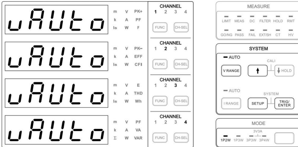
Figure 4-20 Voltage Range Setup Screen
