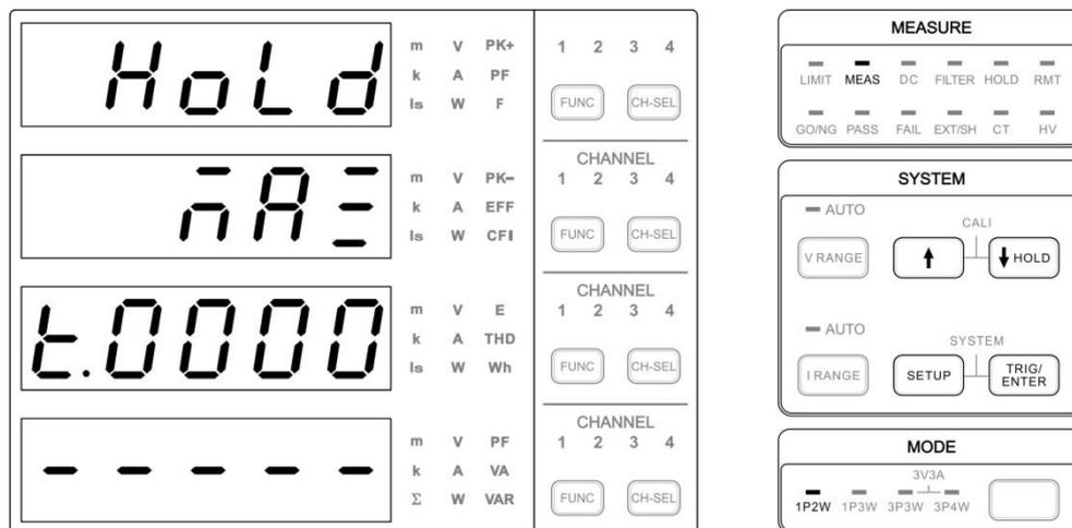
Figure 4-49 HOLD Setup Screen
