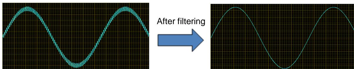
Figure 4-45 Before and After Waveform Filtering
