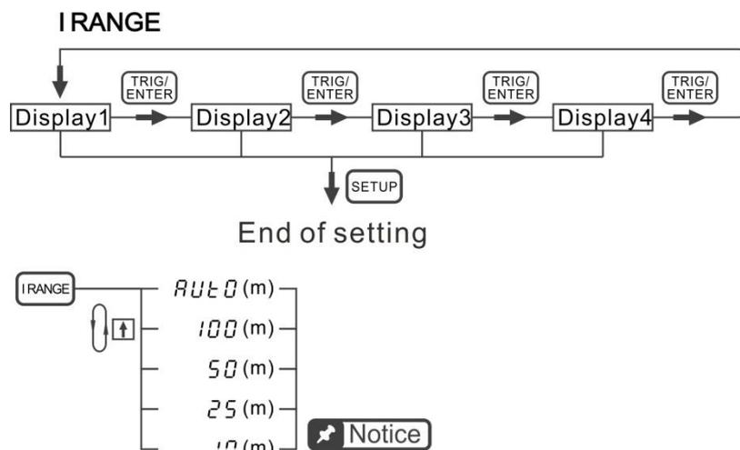
Figure 4-29 Process for Setting Current Range External
