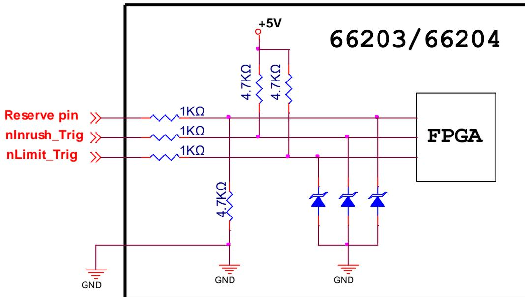
Figure A-1 Limit\_Trigger & Is\_Trigger Internal Wiring Diagram
