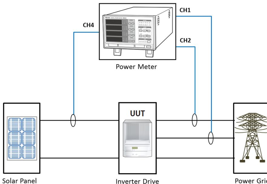
Figure 4-11 Wiring Diagram of 66203/66204 & Converter for Efficiency Test
