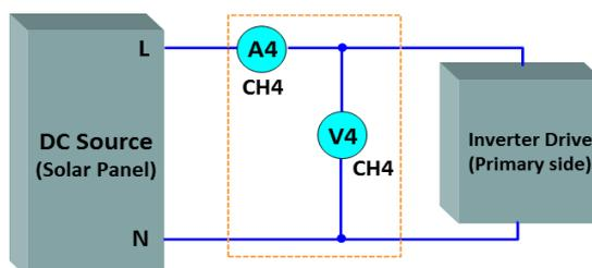
Figure 4-12 Input Wiring of 66203/66204 & Converter for Efficiency Test
