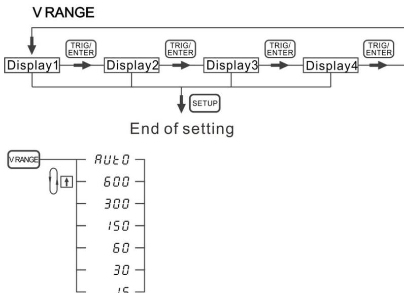
Figure 4-22 Process for Setting Voltage Range
