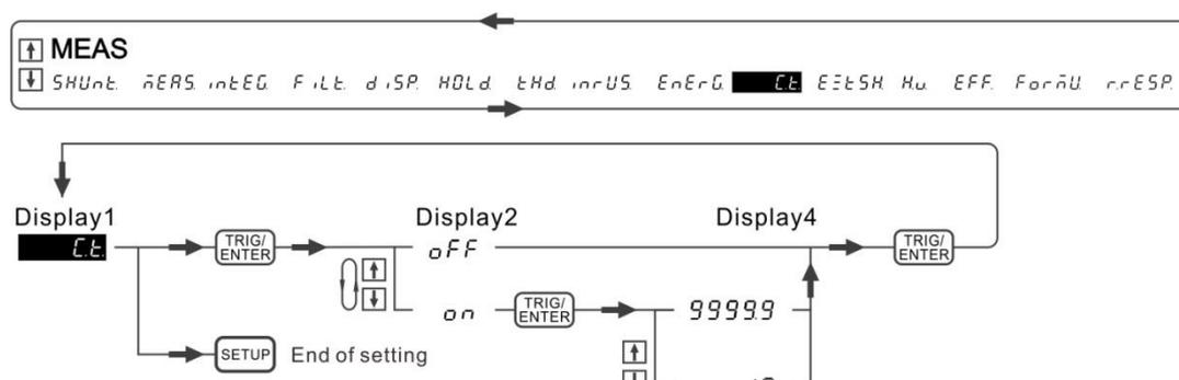
Figure 4-62 Process for Setting CT
