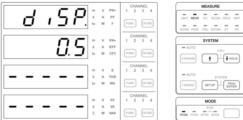
Figure 4-47 DISPLAY Refresh Rate Setup Screen
