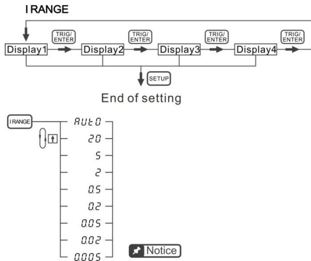
Figure 4-15 Process for Setting Current Range
