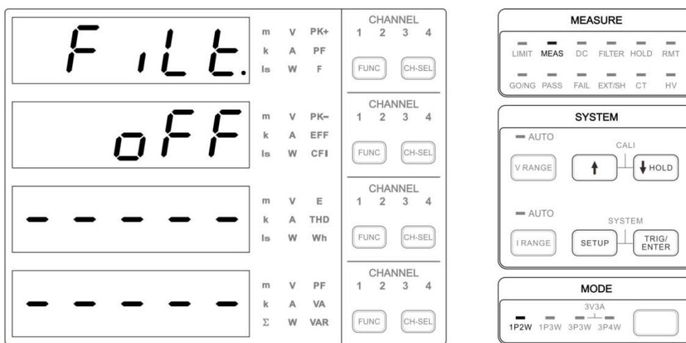
Figure 4-44 FILTER Setup Screen
