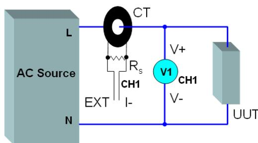
Figure 4-61 CT Wiring for EXT & I-
