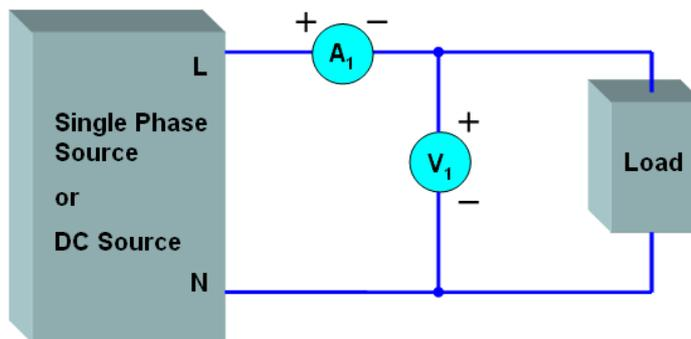
Figure 4-77 1P2W Wiring Diagram
