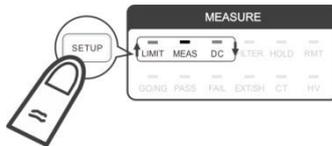
2. Use  $\uparrow$ ,  $\downarrow$  to select Formu function in the 1<sup>st</sup> display window and press **TRIG/ENTER** to confirm it.
