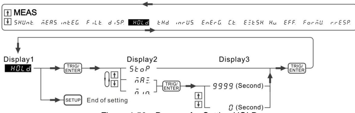
Figure 4-50 Process for Setting HOLD
