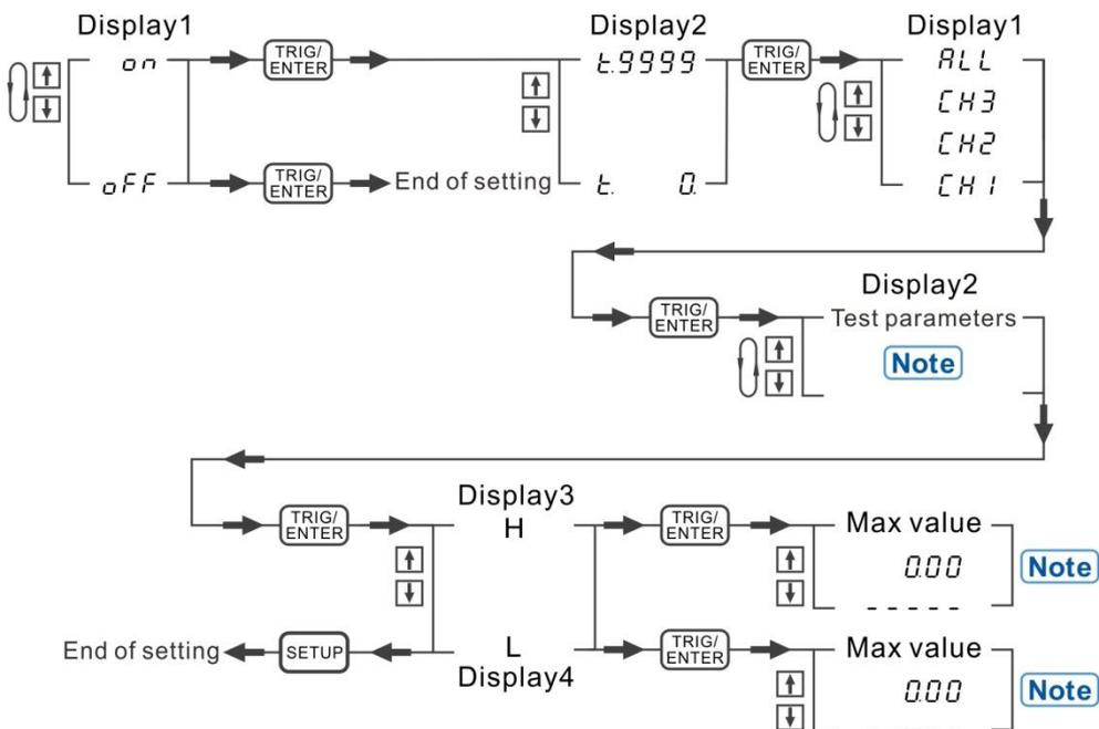
Figure 4-31 Procedure for Setting Limit Function
