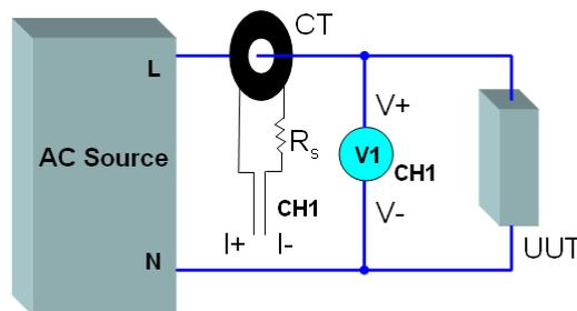
Figure 4-60 CT Wiring for I+ & I-
