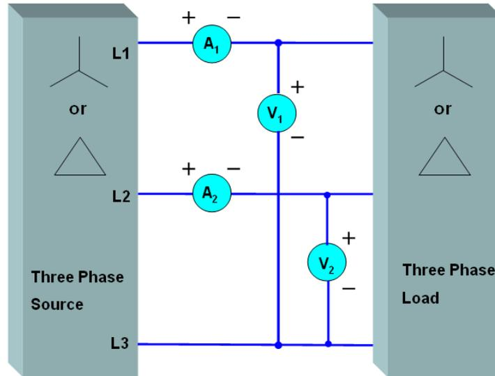
Figure 4-79 Two-Wattmeter Method Diagram
