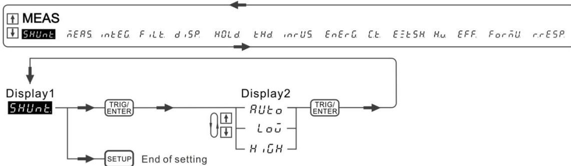
Figure 4-37 Process for Setting Shunt
