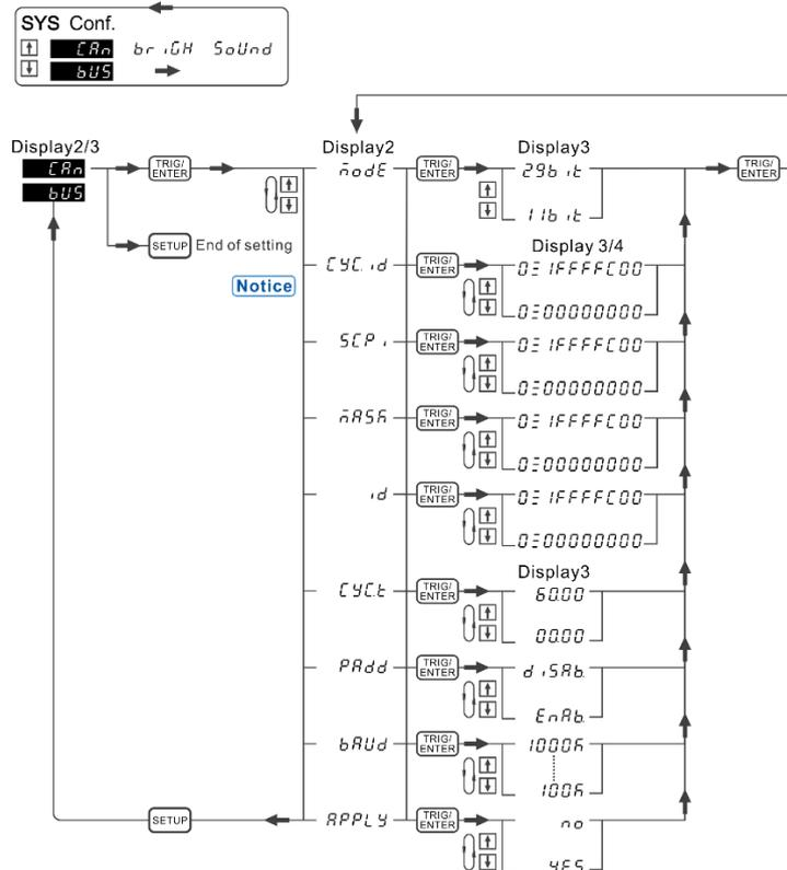
Figure 4-6 Process for Setting CAN bus
