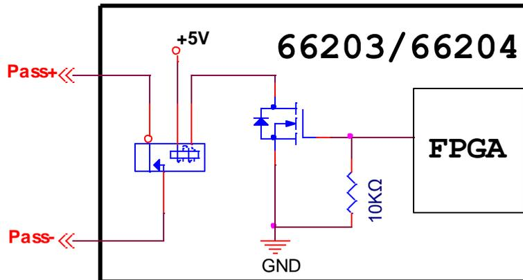
Figure A-2 Pass + / Pass – Internal Wiring Diagram
