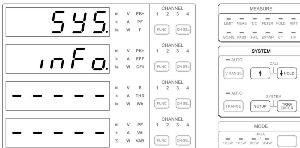
Figure 4-1 Menu for Checking Firmware & Digital Version
