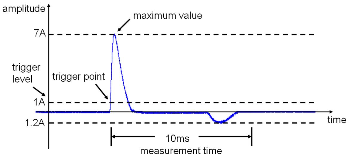
Figure 4-56 Example of Inrush Current Measurement
