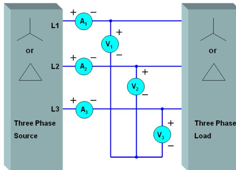
Figure 4-81 Three-Wattmeter Method Wiring
