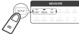
2. Use **↑**, **↓** to select Meas. in the 1<sup>st</sup> display window and press **TRIG/ENTER** to confirm it.
