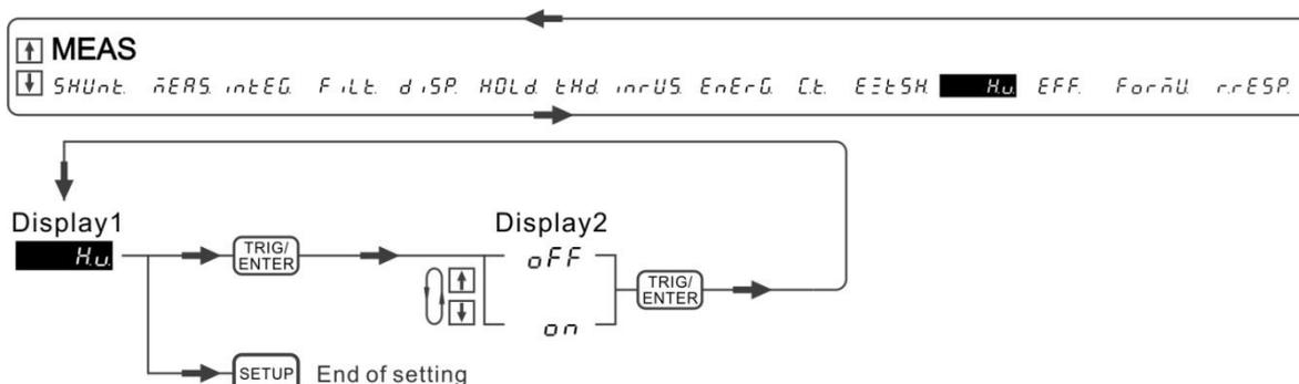
Figure 4-68 Process for Setting HV (when firmware version is < 1.21)
