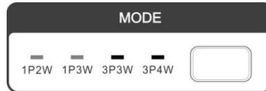
2. If the actual connection does not match the measurement mode, the PF measurement could be larger than 1, the display will show PF over range warning (Over Power Factor Range, OPFR). It is only supported when the firmware version is  $\geq 1.21$ .
