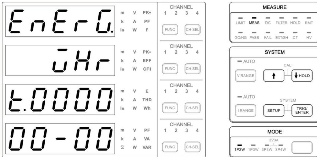
Figure 4-57 ENERGY Setup Screen
