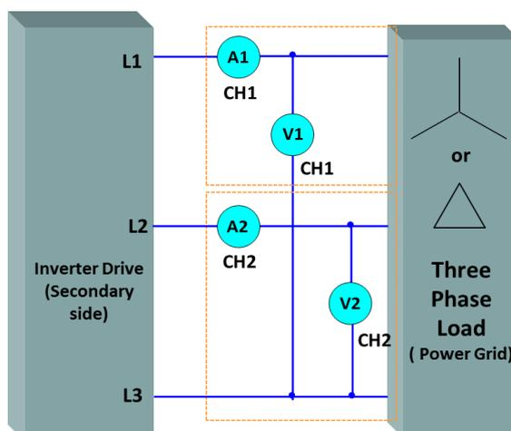
Figure 4-13 Output Wiring of 66203/66204 & Converter for Efficiency Test
