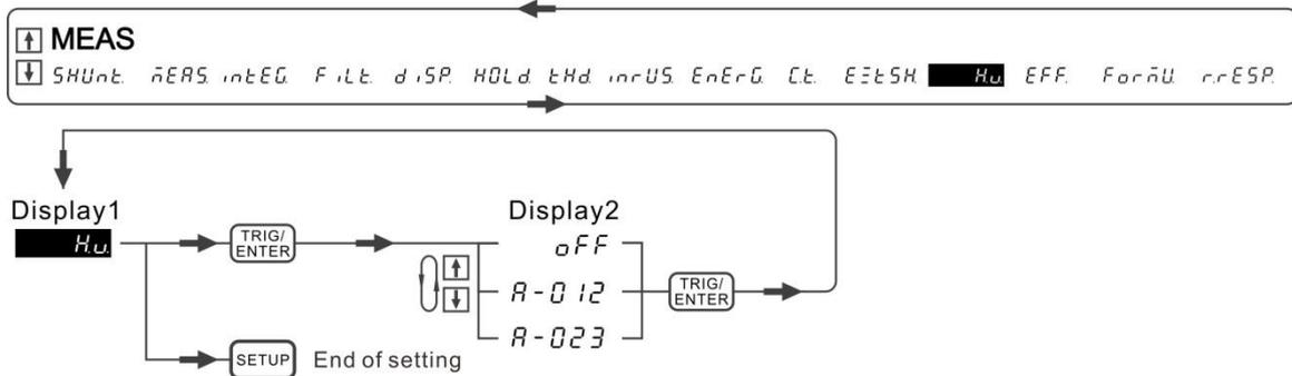
Figure 4-69 Process for Setting HV (when firmware version is  $\geq 1.21$ )
