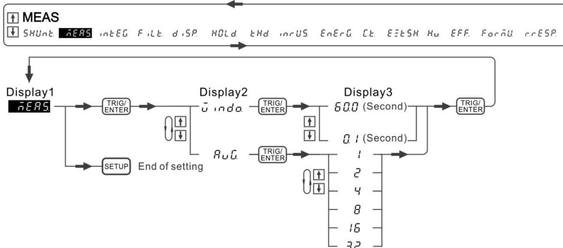
Figure 4-40 Process for Setting WINDOW & AVG Measurement Functions
