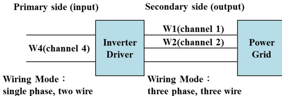
Figure 4-10 Power Meter Configuration for Testing Converter's Efficiency
