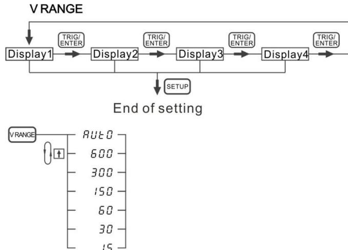
Figure 4-14 Process for Setting Voltage Range
