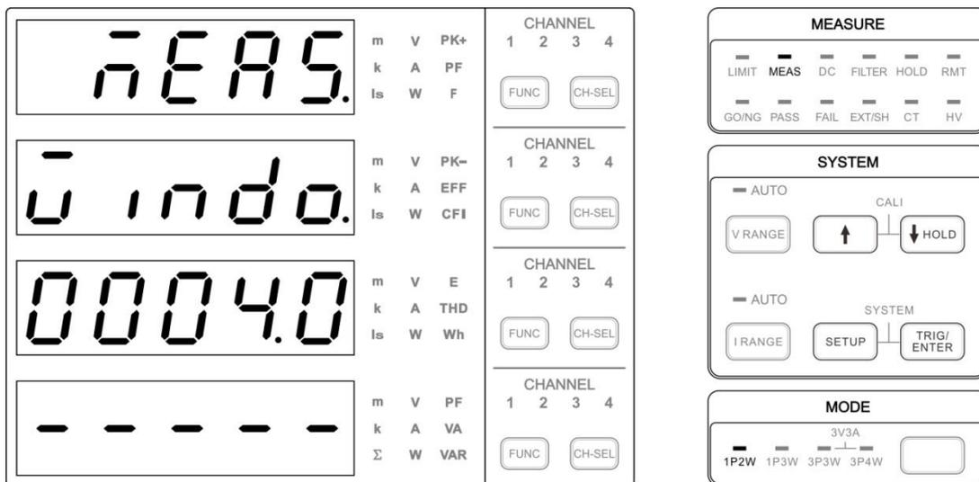
Figure 4-38 WINDOW Measurement Setup Screen
