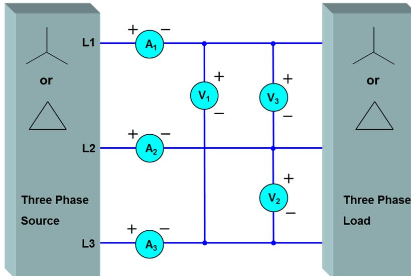
Figure 4-80 Three-Wattmeter Method (3V3A) Wiring
