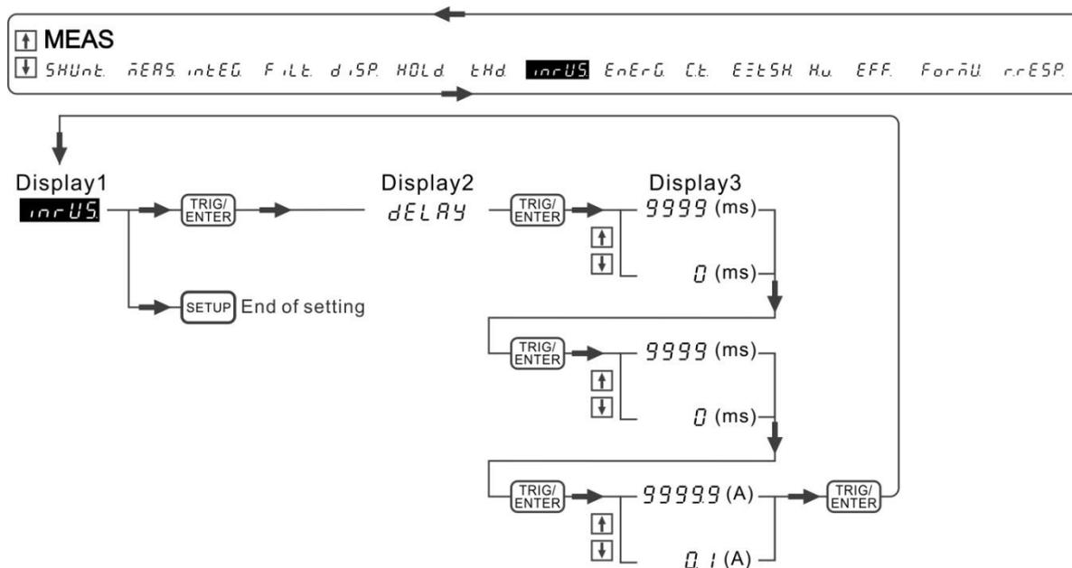
Figure 4-55 Process for Setting INRUSH CURRENT
