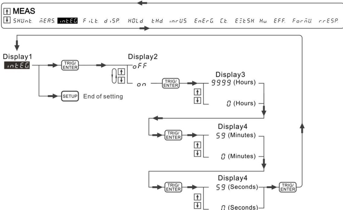
Figure 4-42 Process for Setting Integration
