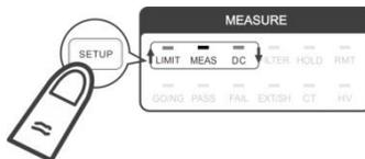
2. Use **↑**, **↓** to select inrUS in the 1<sup>st</sup> display window and press **TRIG/ENTER** to confirm it.
