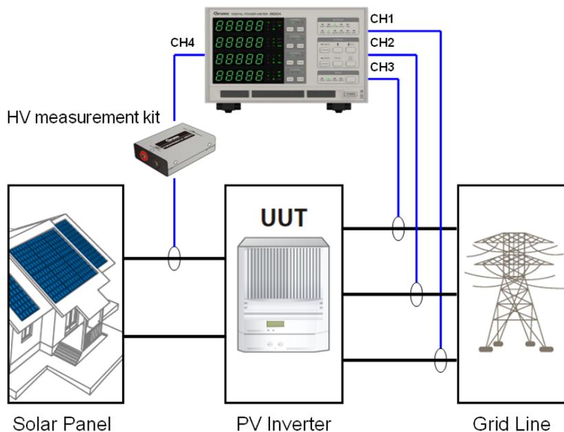
Figure 4-67 HV Measurement Kit Wiring Diagram
