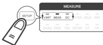
2. Use **↑**, **↓** to select Meas. in the 1<sup>st</sup> display window and press **TRIG/ENTER** to confirm it.
