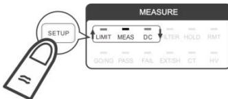
2. Use  $\uparrow$ ,  $\downarrow$  to select EFF function in the 1<sup>st</sup> display window and press **TRIG/ENTER** to confirm it.
