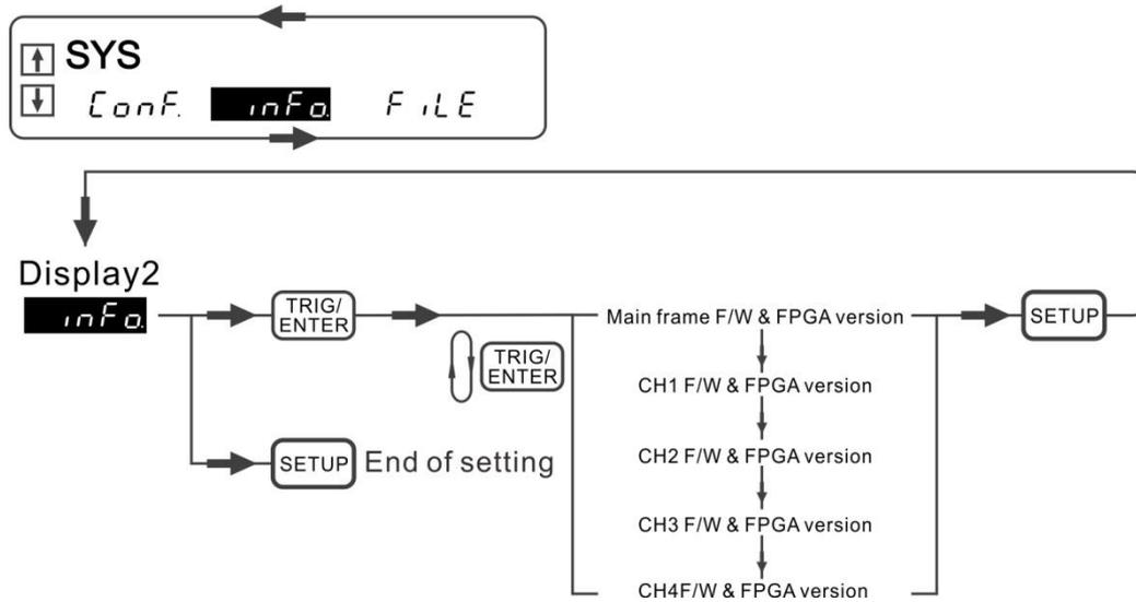
Figure 4-2 Process for Checking Firmware & Digital Version
