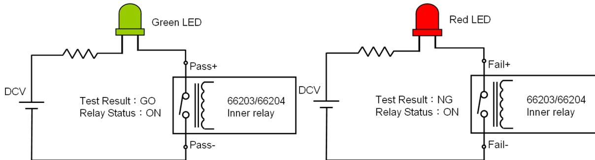
Figure 4-35 Wiring of GO/NG External Indicator
