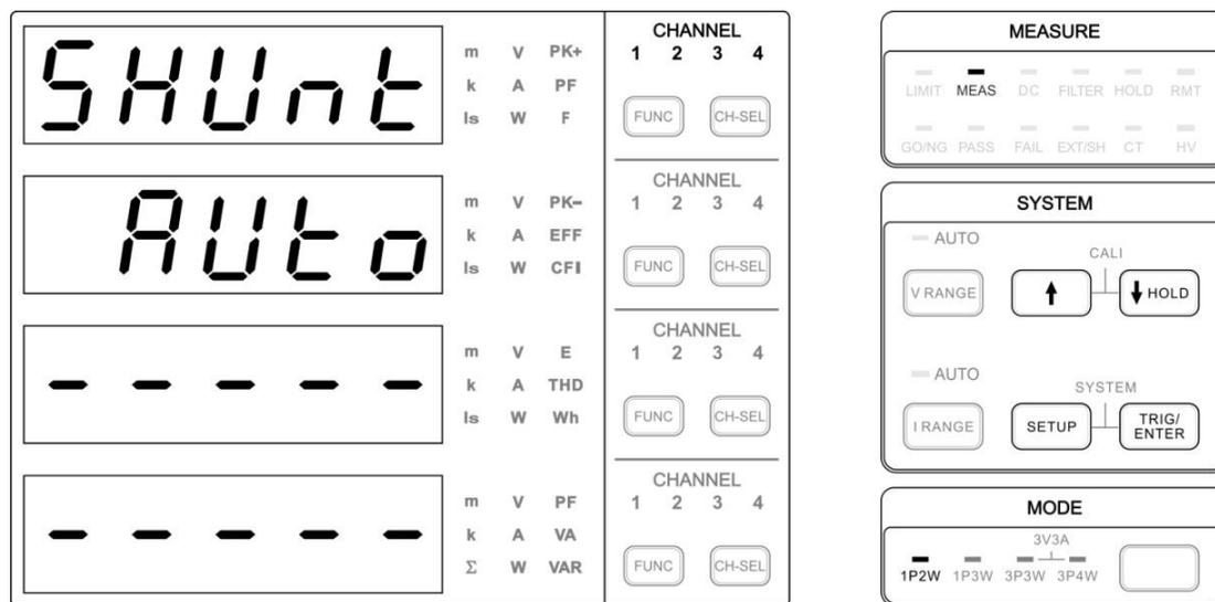
Figure 4-36 Setup Screen of SHUNT
