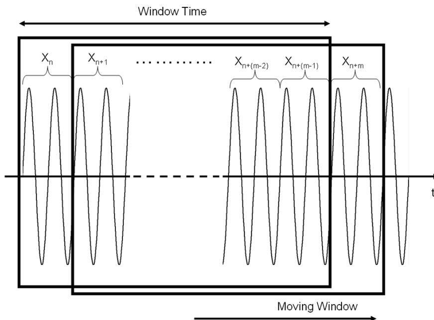
Figure 4-39 WINDOW Measurement Theory
