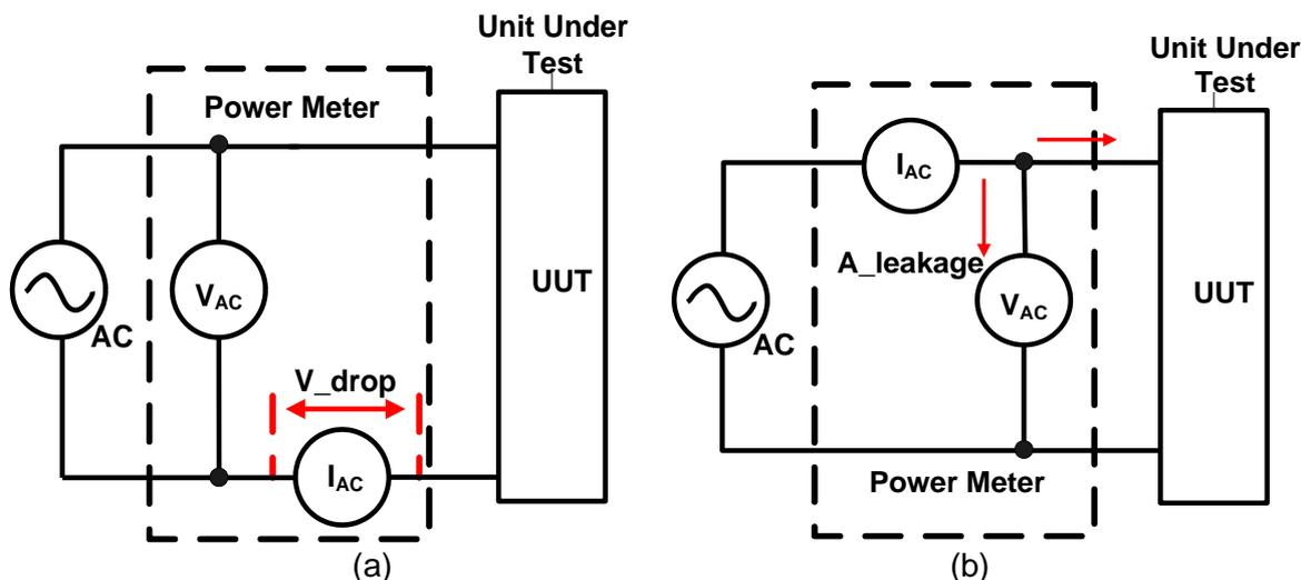
Figure 4-9 Measurement Theory for Power Meter Connection
