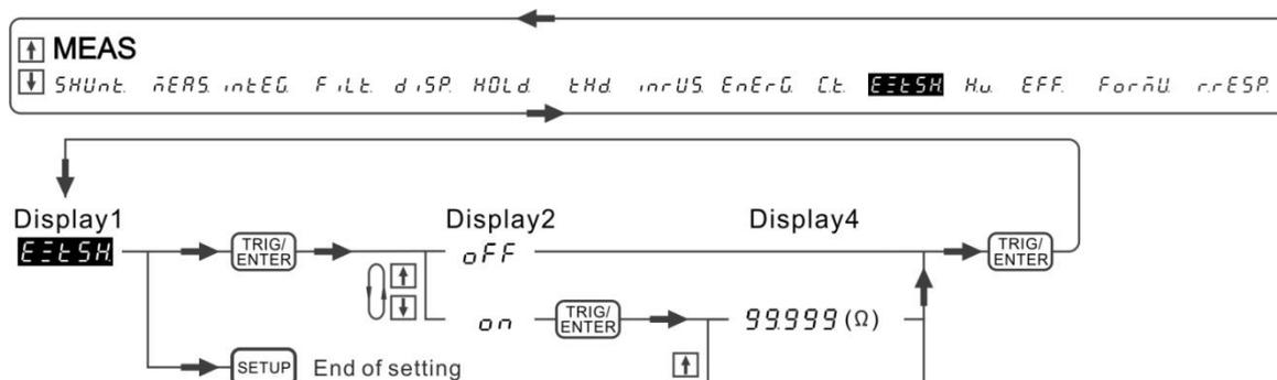
Figure 4-65 Process for Setting ExtSH
