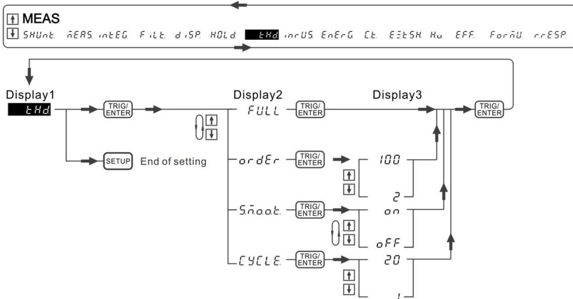
Figure 4-53 Process for Setting THD
