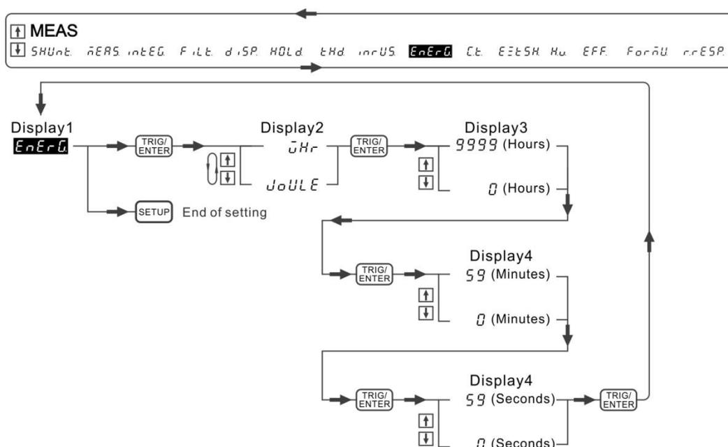
Figure 4-58 Process for Setting ENERGY
