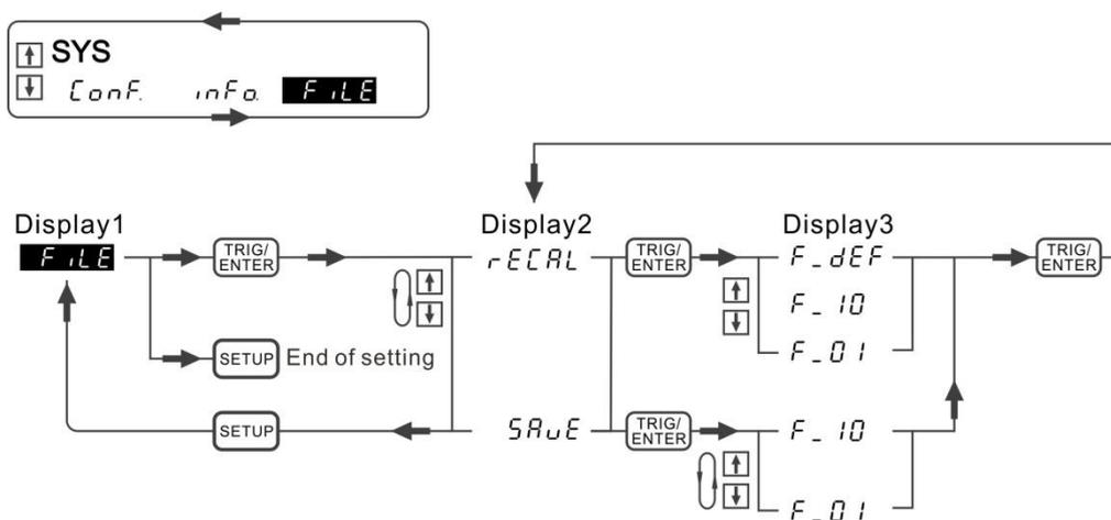
Figure 4-8 Process for Saving & Recalling Setting File
