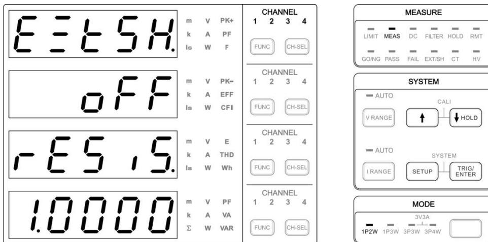
Figure 4-63 EXTERNAL Setup Screen
