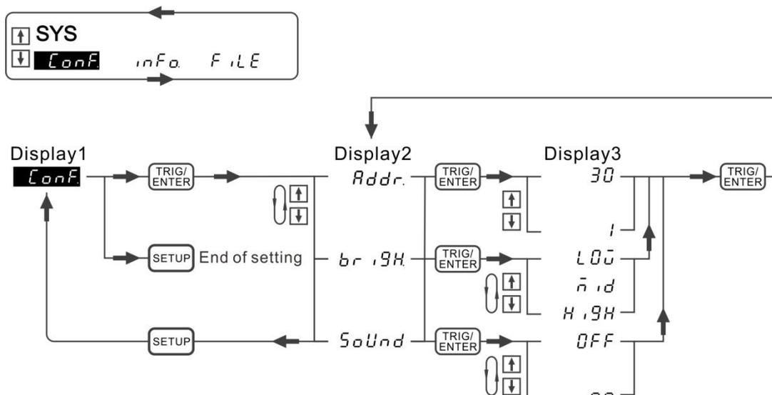
Figure 4-4 Process for Setting Communication Address, Display Backlight & Sound
