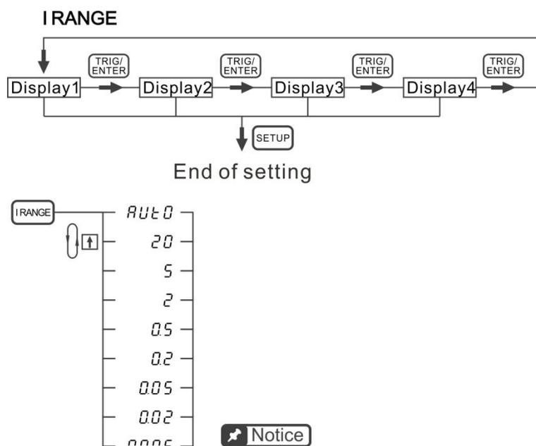
Figure 4-26 Process for Setting Current Range
