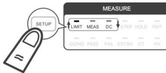
2. Use **↑**, **↓** to select on in the 1<sup>st</sup> display window and press **TRIG/ENTER** to confirm it.
