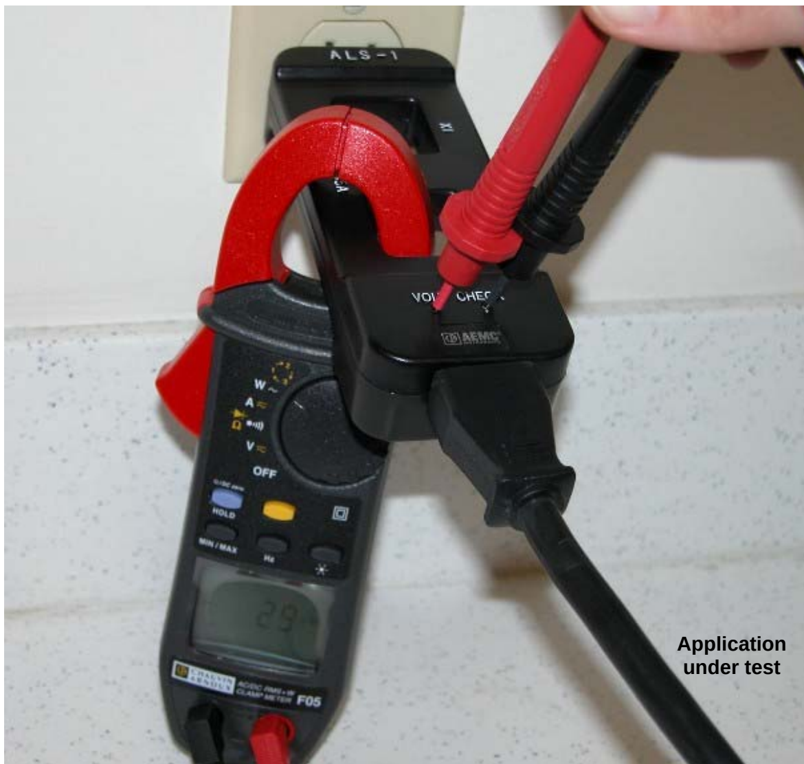
Figure 1 – Using a Clamp-on Meter with the AC Line Splitter Model ALS-1
