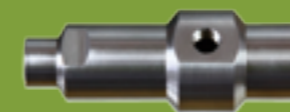
SH-PP - Flow chamber for compressed air measurement up to 25 bars - stainless steel DIN 1.4301 inlet and outlet connection - G1/8 thread humidity probe connection - G1/2 thread screw-coupling not included.
