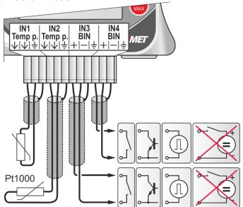
For the procedure for connecting wires to the connecting block refer to Annex 4.
