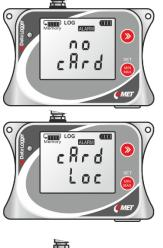
Displayed when no SIM card is inserted
