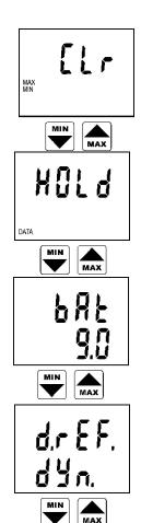
Clearing of minimum and maximum memory of all values. Memory is cleared after pressing ENTER key. Clearing is confirmed by reading YES on the LCD lower display.
