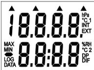
Connect the external probe to the connector before switching ON the instrument. Switch ON the instrument by pressing ON/OFF key. After switching ON the instrument all symbols on the LCD are displayed. If the ON/OFF key is being held pressed, all LCD symbols are displayed till the key is released.
