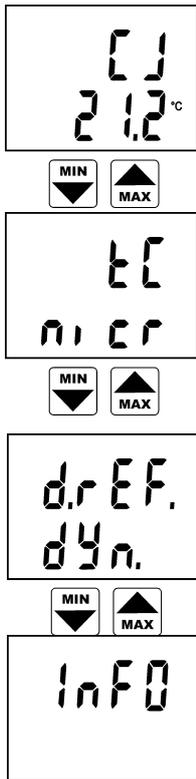
Type of actual selected thermocouple is indicated - symbols **J** or **nicr** (K thermocouple) or **S**. Press ENTER key to enter the thermocouple selection mode (procedure is described below). If the selection is not correct. temperature readings are incorrect.
