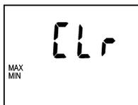
Clearing of minimum and maximum memory of temperature. Memory is cleared after pressing ENTER key. Clearing is confirmed by reading YES on the LCD lower display.
