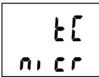
Actual selected thermocouple type is then displayed shortly. Symbols J or n1c (thermocouple K) or S indicate actual thermocouple type. If selected thermocouple does not match the probe type connected to the instruments, temperature readings will not be correct and new selection of thermocouple type is necessary (see below).
