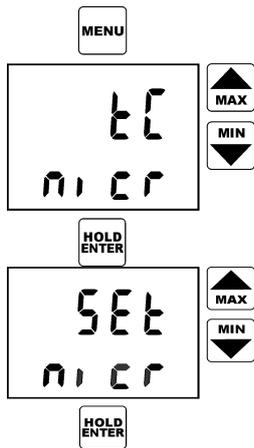
Select menu item tC to select thermocouple type. Confirm the desired thermocouple type by pressing ENTER.
