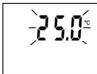
It is possible to set lower and upper limit for measured temperature. Breaking of the limit is indicated by blinking of the value on the display. Alarm activation can be disabled by setting lower alarm limit up to its maximum. This is indicated by OFF reading at the position of numeric value. Value of upper limit of the same alarm is indifferent.
