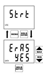
If it is needed to clear the memory before logging start, first it is necessary to select menu item logging START (symbol Strt) and confirm by pressing ENTER key.
