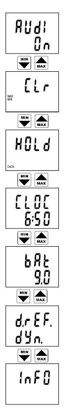
This item indicates if audio signaling of alarm indication is switched on (On) or switched off (OFF). Press ENTER key to change actual setting. Notice: if the battery voltage is low, audio indication is out of operation to reduce current consumption independently on this selection.
