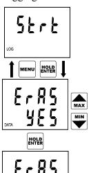
If it is needed to clear the memory before logging start, first it is necessary to select menu item logging START (symbol Strt) and confirm by pressing ENTER key.
