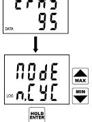
Clearing procedure is in progress. It takes approximately 16 s and the duration is indicated by displaying of already cleared memory in % (digits 0 to 100).
