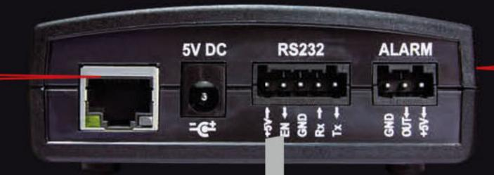
To communicate with a PC and other systems, the device is equipped with a USB port (located on the side of the device), RS232 and Ethernet.
