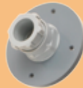
SH-PP - Flow chamber for compressed air measurement up to 25 bars - stainless steel DIN 1.4301 inlet and outlet connection - G1/8 thread humidity probe connection - G1/2 thread screw-coupling not included.
