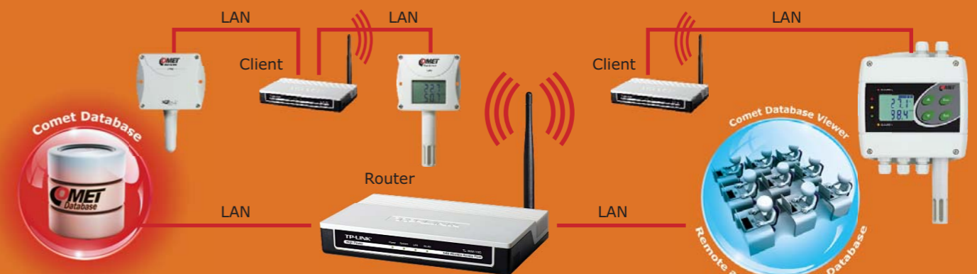
TP-LINK-TL Wi-Fi adapter for wireless connection of transmitter or data logger to Ethernet network. Including replaceable antenna and power adapter. Long term proved operation.
