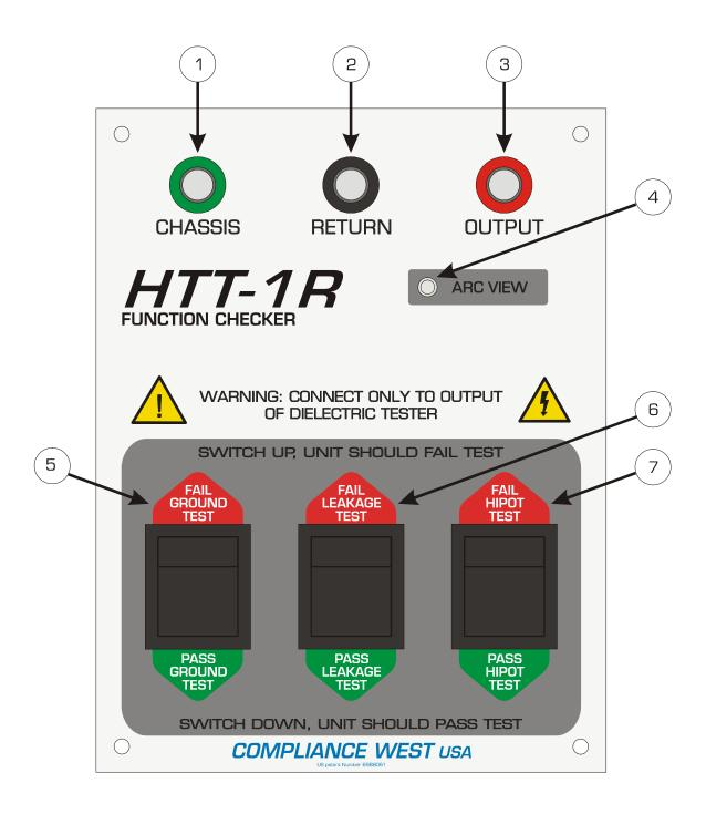
Figure 1: HTT-1R Front Panel Features
