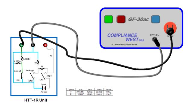
Figure 3: Connection to a Ground bond tester
