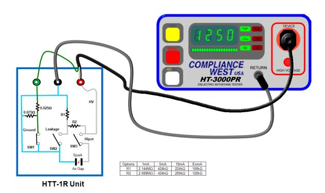
Figure 2: Connection to a hipot tester
