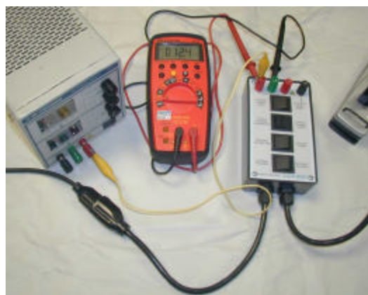
Figure 11 Leakage Test - Isolated
