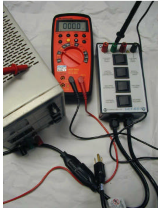
Figure 1 Grounding Circuit Continuity Test
