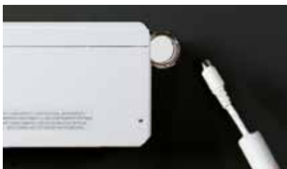
Opening to run cable to finger touch unit
