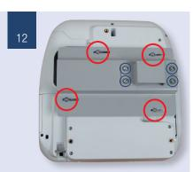
Carefully place the projector plate on top of the spacers and washers and secure the plate with  $4 \times 45$  (0.15"  $\times 1.8$ ").
