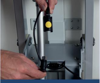
Put the plug of the external actuator into the connector marked with the yellow dot.
