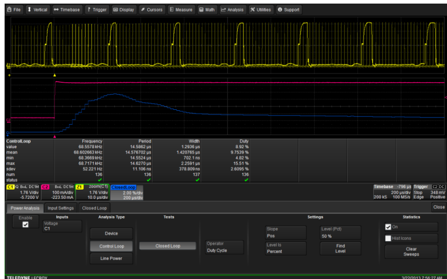
Figure 1: Measuring the step load response in a switched mode power supply using Teledyne LeCroy's Power Analysis option software
