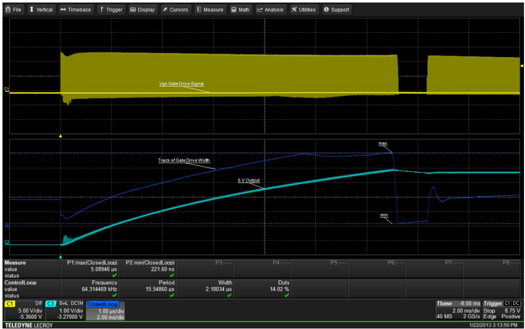
Figure 2: A control loop study showing the startup of the power supply
