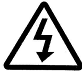
Danger!: High voltage
