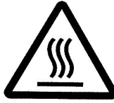
Danger!: High temperature
