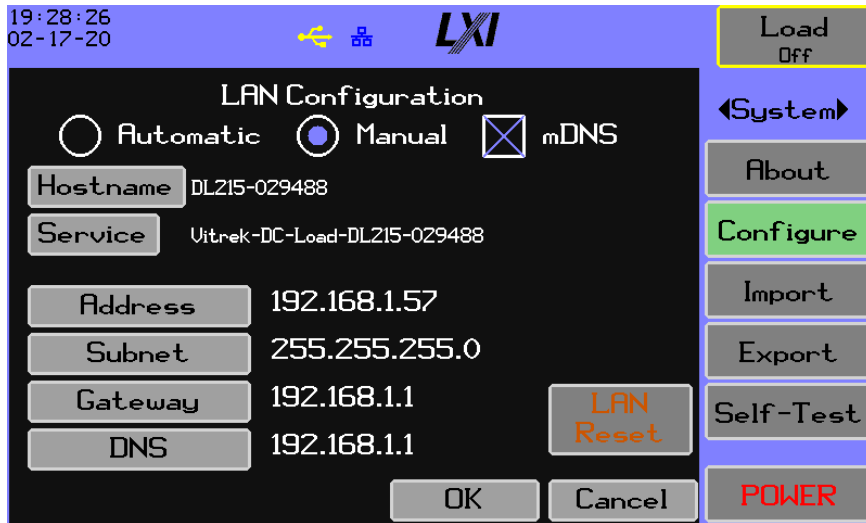
Figure 5-55 LAN Configuration – Manual Setting
