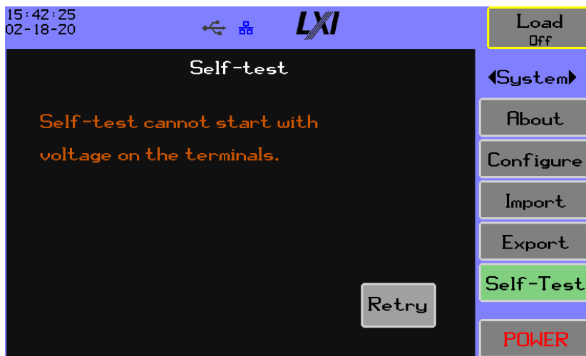
Figure 5-60 Self-test Cannot Start
