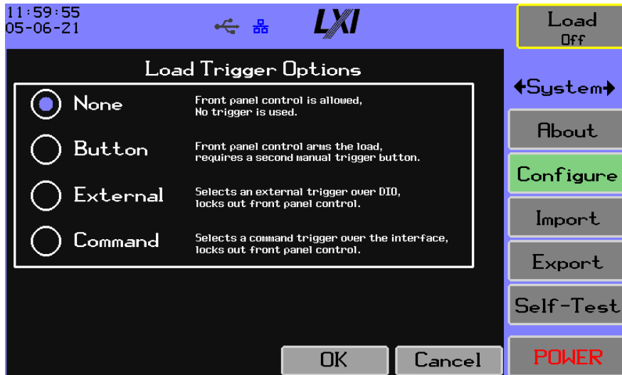
Figure 5-56 Load Trigger Options
