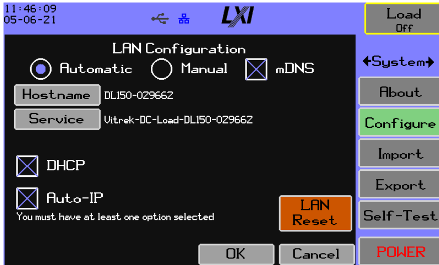
Figure 5-53 LAN Configuration Screen
