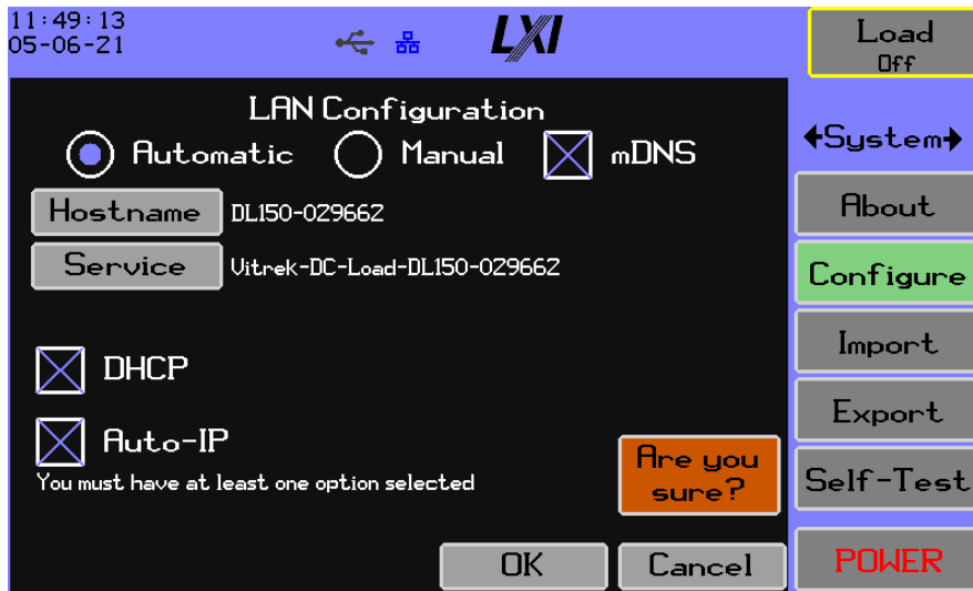
Figure 5-54 LAN Configuration Factory Reset Confirm
