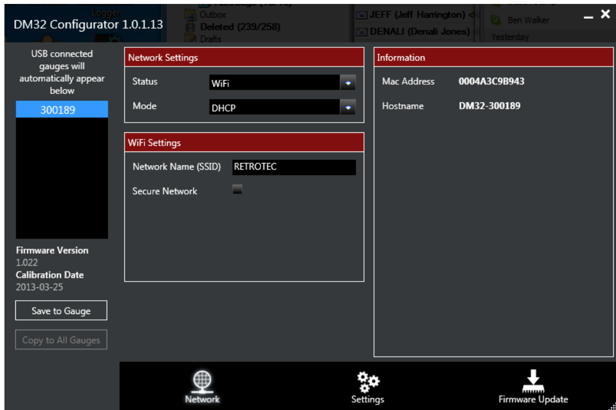
Figure 18: Non-secure WiFi needs DHCP and Network name entered
