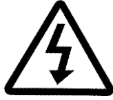
Danger!: High Voltage
