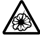
Danger!: Explosion Hazard
