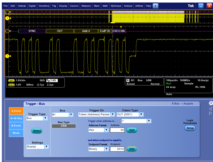
Triggering on a specific PID on a USB full-speed bus. A complete set of triggers, including triggers for specific token (address) and data packet content, ensures you quickly capture your event of interest.
