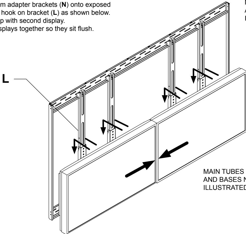
**10** Hook one top adapter bracket (**M**) onto exposed threads on hook on bracket (**L**) as shown below. Repeat step with second display.
