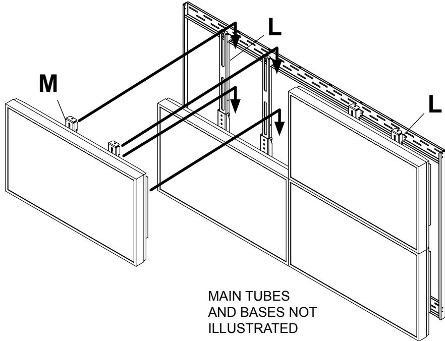
**11** Secure top adapter brackets (**M**) to hook on brackets (**L**) using four M5 x 10 mm socket pin type-F screws (**R**) as shown below.
