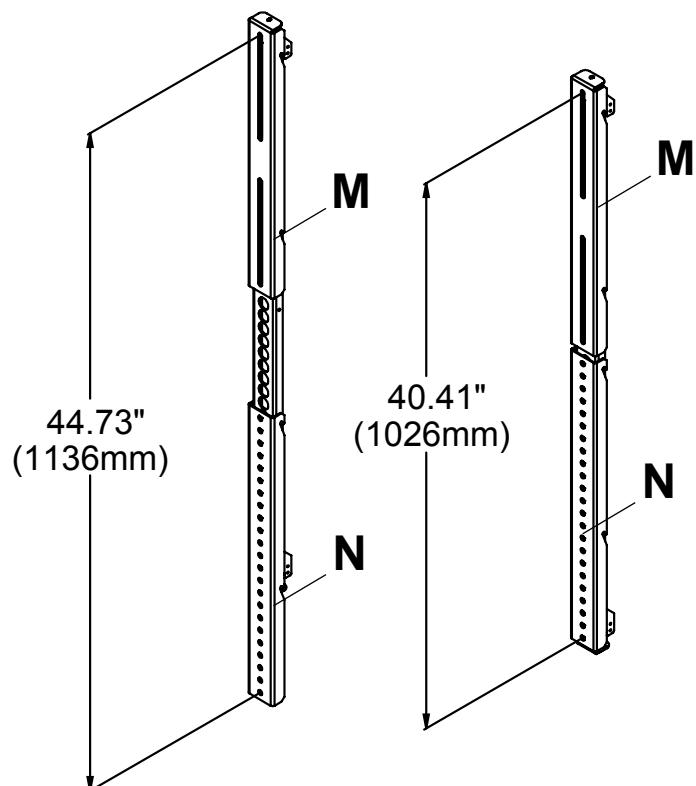
**5** Hook one the bottom adapter bracket (**N**) onto the exposed threads on the hook on bracket (**L**) as shown below. Hook one the top adapter bracket (**M**) onto the exposed threads on the hook on bracket (**L**) as shown below.
