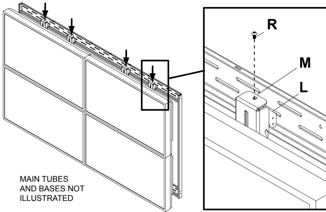
**12** Once displays are in desired position, secure using four security screws located on bottom of hook on brackets (L).
