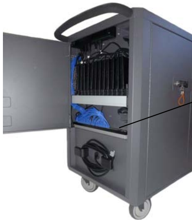
Network cables and Cisco switch pre-installed
