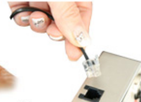
The sensor loop plugs into the alarm module. Cutting or unplugging triggers the alarm
