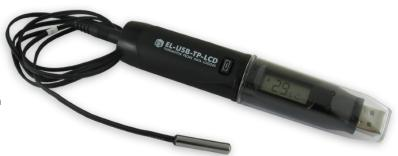
This standalone data logger measures and stores up to 32,510 temperature readings from the supplied high accuracy thermistor probe which is attached via the socket at the base of the unit. The user can easily set up the logging rate and start-time, and download the stored data by plugging the data logger into a PC's USB port and running the purpose designed software under Windows XP, Vista, 7 or 8. Data can then be graphed, printed and exported to other applications.
