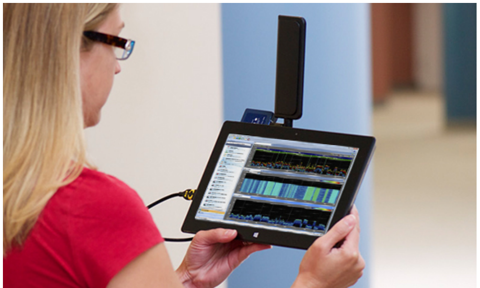
AirMagnet Spectrum ES can scan frequencies between 698 MHz and 2690 MHz and includes support for multiple technologies.
