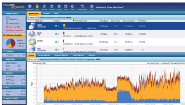
The Performance Bottleneck Analysis function of the NTM V8.0 shows the average time application flows (for example, SMTP and HTTP) spent on the server and network. The bottom graph area indicates a sudden increase and return to normal in server time during the analysis period.
